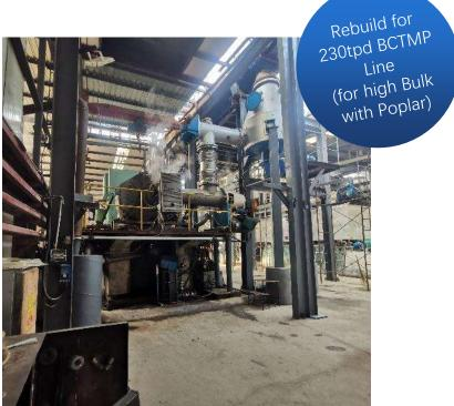
Yunda replaced the whole Impregnation System with MSD by Yunda Thermal Shredding System,
